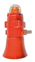
The phone signal Ex-Duo signalises incoming calls from stationary telephones as a secondary ringing device. The signaling is ensued by a 5 joules flash and by a 110 dB(A) sounder. Once an incoming call is signalised, the flash and the sounder will be activated. Between the ringing signals the flash is bridged for continuous flashing. Different sounds can be set individually.
