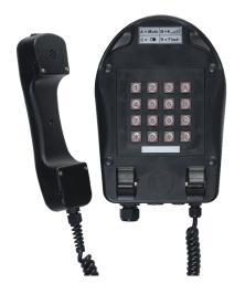
The lightweight Ex industrial dA24 telephone is designed for explosion prone areas. It can be used as a PABX device and end device as well as for DTMF or pulse dialling. In the event of loud environmental noise, you have the option of turning on an integrated handset amplifier. A continuously adjustable fixture protects the telephone handset against shocks. The robust 16-part keypad can also be ordered with lighted keys. Upon request, we can also supply the dA24 with two self configurable keys.
